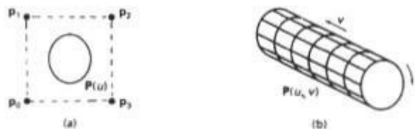
Figure 10-53 Constructing a solid with a translational sweep. Translating the control points of the periodic spline curve in (a) generates the solid shown in (b), whose surface can be described with point function P(u, v) .
